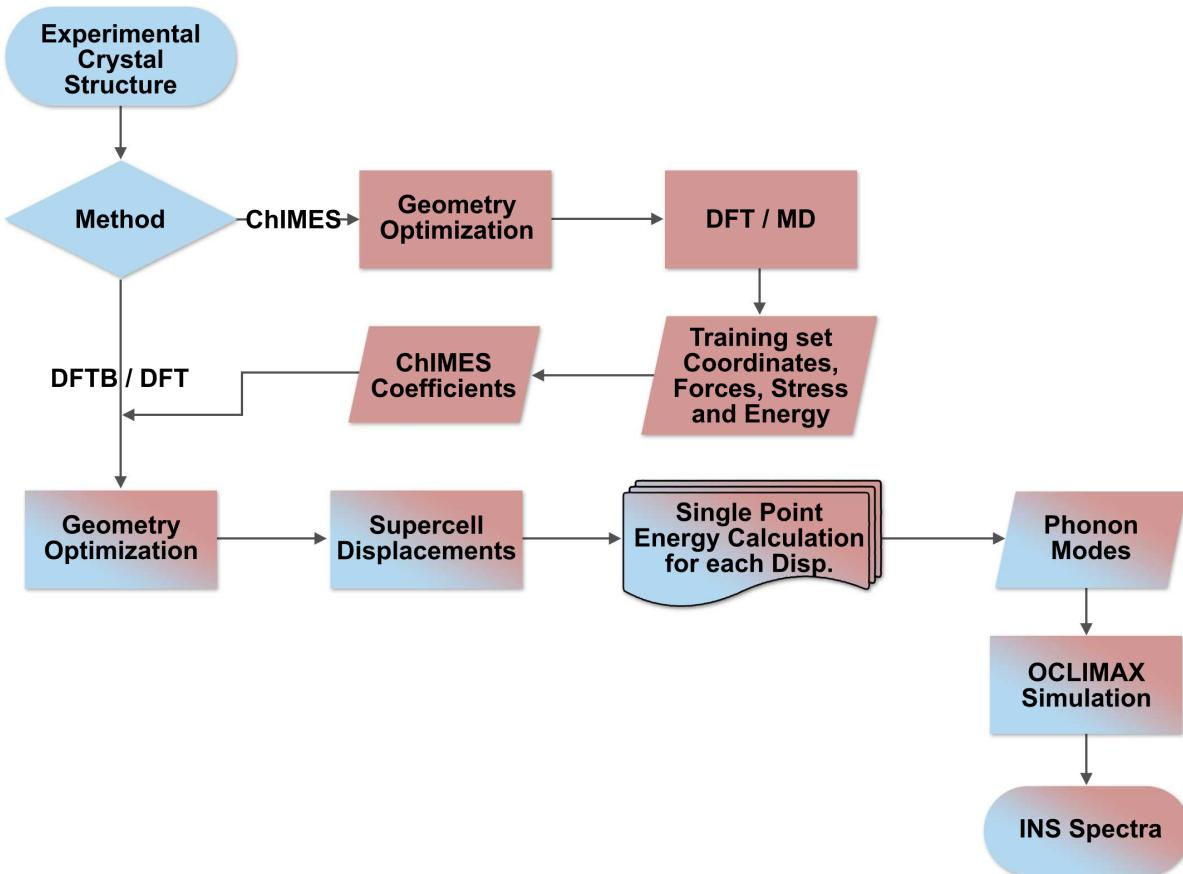
In the figure above, we present an overview of the complete workflow of the DCS-Flow method. The main part of it is composed by steps in blue or that contain a blue gradient. With the experimental crystal structure file and a set of workflow parameters as inputs, we optimize the structure, simulate the lattice dynamics with the supercell method and calculate the INS spectrum. This is called the main workflow.
